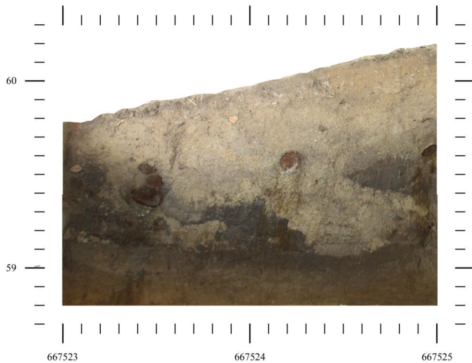
Figure 5.5. Bates #2, TU-1, north profile. Key: (F1) gray clay fill; (F2) heavily basket-loaded fill; (A) buried A-horizon; (E) E-horizon; (B) Bt-horizon; areas of bioturbation are shaded gray.
